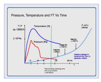
An arc is accompanied by radiation in the form of light, sound, and heat. Therefore, the presence of an arc can be detected by analyzing visible light, sound waves, and temperature change.
